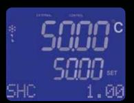
For further optimization of temperature control, you can easily input the specific heat capacity value for the heat transfer fluid that you're using.
