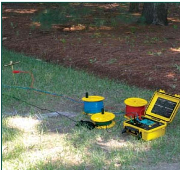
*The Model 6472 performs an automated way to measure the value of the earth/ground using the Fall-of-Potential method and storing measurements.*
