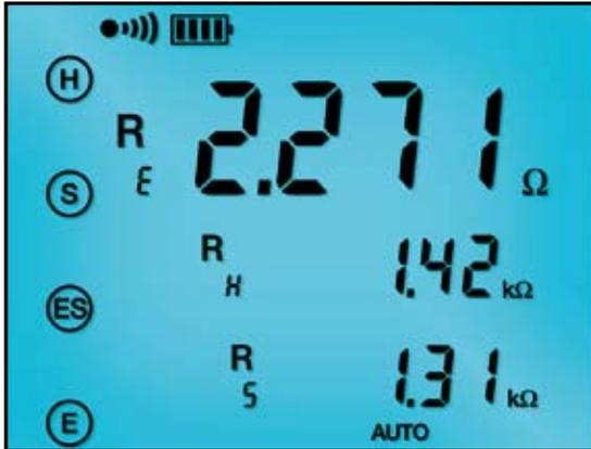
The 4-Point Bond test displays lead connections, bond resistance test results, test voltage and current.
